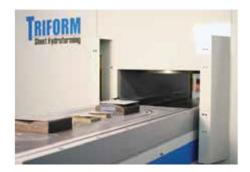
A series of five different fluid cell tools rests unsecured on a sheet hydroforming press table. Benefits of the fluid cell sheet hydroforming process include the ability to run multiple different parts in a single press cycle.
