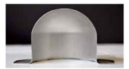
A deep drawn part cross section shows uniform wall thickness. Because the material is wrapping around the punch tool as it is raised into the diaphragm, material is elongated more uniformly when compared to traditional drawing methods.
