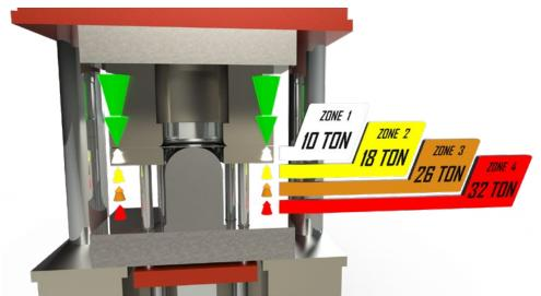
Beckwood's Dynamic Cushion Control allows Columbia Metal Spinning to adjust the tonnage of the bed cushion throughout four travel zones for greater control over material flow.
